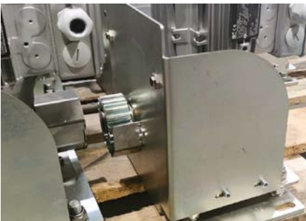
Dust and snow protection for the cabinet.
